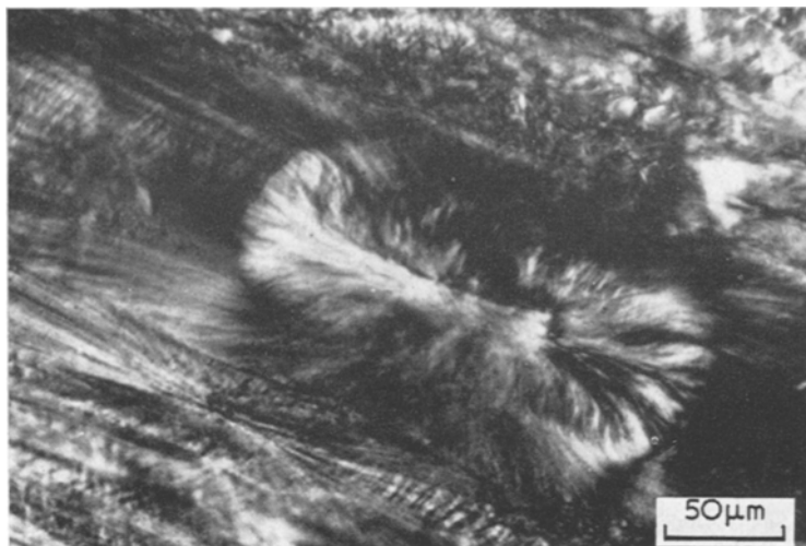
Figure 2 Highly-deformed ringed spherulite.
